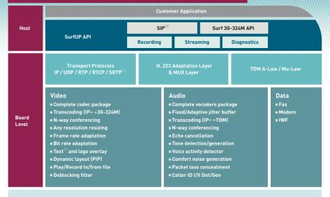
The system architecture used in the SurfRider-812/PTMC is optimized to reduce bottlenecks.
