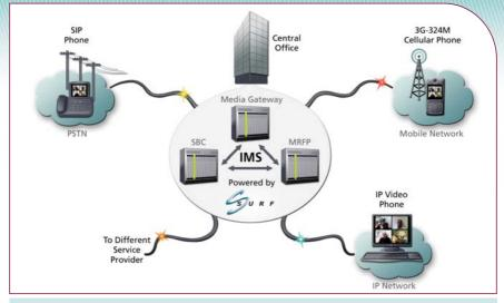
Typical network topology illustrating how the SurfRider-812/PTMC DSP resource card integrates into network infrastructure equipment to enable convergence of Voice + Video + Data across Wireline and Wireless networks.
